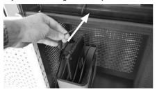
Neatly bundle the excess cable in the charge compartment. The power strips can be slid along the track to create space.
