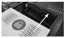
Plug the Carrier 10 Charging Station power cable into the unit, then into the wall socket. Charging will commence automatically (may need to switch the wall outlet "on").
