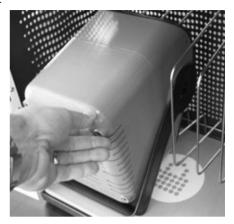
If you have devices that can fit in the plastic baskets, remove the Stainless Steel Device Rack and mat, otherwise leave it in place.
