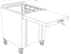
Remove the plastic carry baskets, the mat and the three shelves by lifting on the pull-hole. Lay the shelves on a scratch-proof surface
