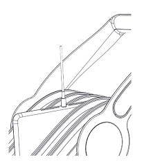
Connect the power cable. Plug cable into cart and into the wall socket\*. The devices will start to charge when power is "On"
