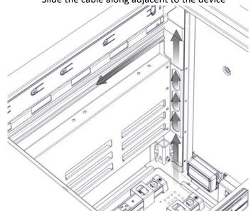
Insert the remaining cables. Evenly space the cables along the rubber grip
